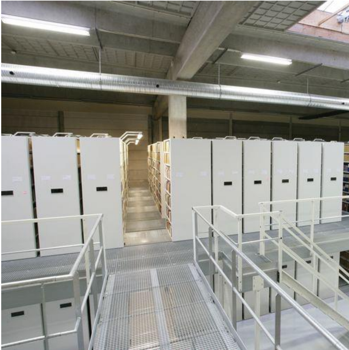
Figure 5: Specialist Archive Standard Double-Decker Mobile Racking for use in the ROLLR Strongroom
